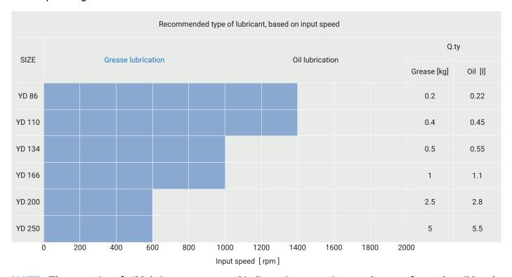
**NOTE**: The quantity of oil lubricant, expressed in litres, is approximate; please refer to the oil level for a correct filling.
