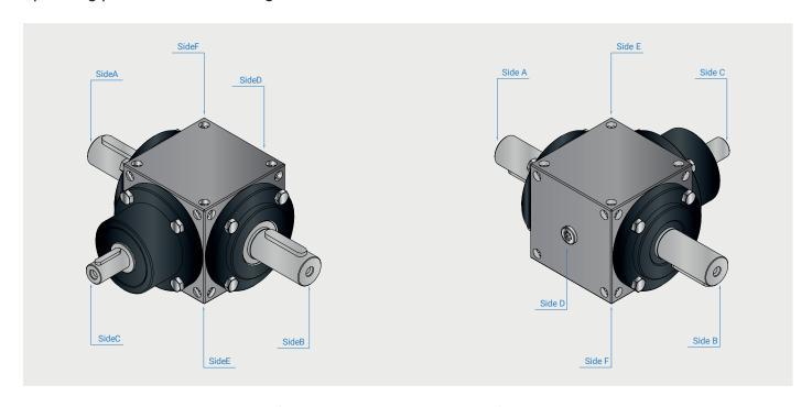
Side C is the side of the main input (solid shaft or IEC motor flange). Side A and side B correspond to the main output axis of the gearbox (solid shaft, cylindrical with key, on one or both sides, or hollow shaft with cylindrical hole and keyway). On side D and / or side E and / or side F it is possible to mount asolid shaft with hub, cylindrical with key, as additional output.
